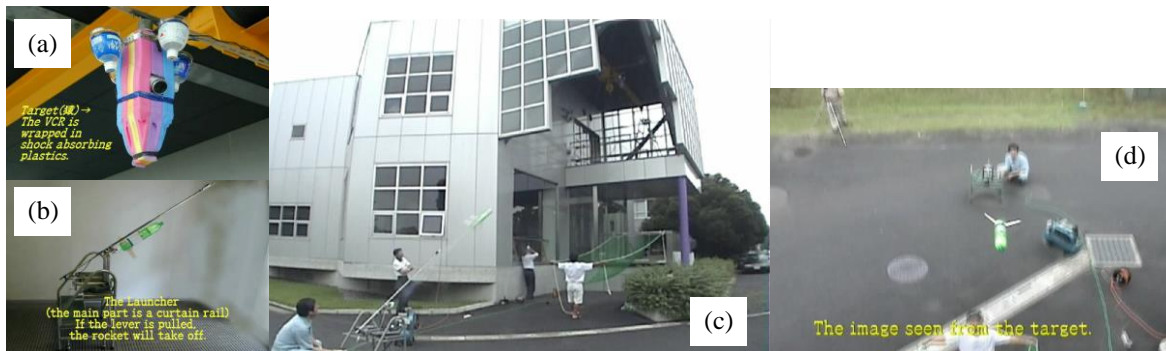
Figure 5. Large device. (a) Falling body, (b) Projectile and launcher, (c) Schematic view, (d) An image of the projectile seen from the falling body
