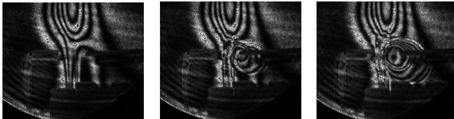
Fig. 4 Still Images from butane combustion by laser interferometer 5,000 fs/s
